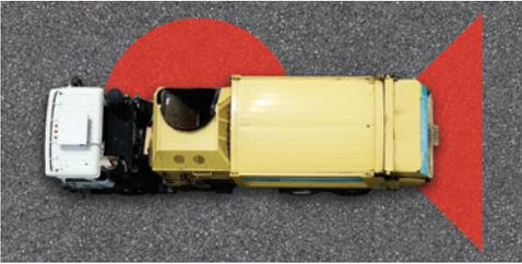
*Rear Load – extends out and away 15 feet from the rear of the vehicle at a 45-degree angle*
